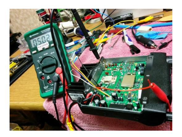
Dan went on to state "The TYT TH9000 has a plastic cover hiding a machined opening to fit a 9 pin serial port, complete with 2 threaded holes to mount a serial port". With this information in hand, I put out a request that I would build the repeater, if someone donated the radios. To my delight, Todd (KD0TLS) and Matt (N0YNT) came forward with the offer of two radios. Matt gave me his TYT-TH9000 and Todd ordered the newer TYT-TH9000D (see his article).
