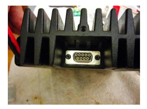
To secure the connector using the threaded holes, I "borrowed" two of the four  $Torx^{TM}$  head screws that held the cover - a perfect fit!
